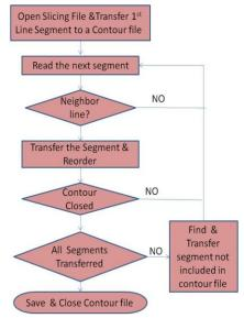
Fig. 5. Contour construction algorithm flow chart.
