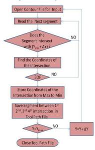
Fig. 7. Flow chart for the contour-filling algorithm
