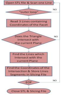
Fig. 4. Slicing algorithm flow chart.
