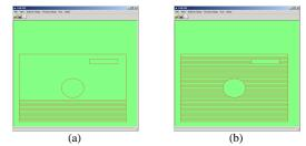
Fig. 11. Raster scan pattern filling.
