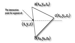
Fig. 3. Three vertices of one triangle and the entersection points.
