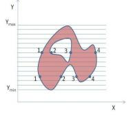
Fig. 6. Contour filling.
