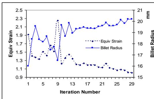
Fig. 7. The Equivalent Strain and Billet Radius vs. Optimization Iteration Number
