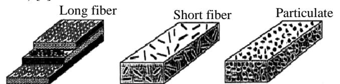
Fig. 2. Types of reinforcement in MMCs [6]
