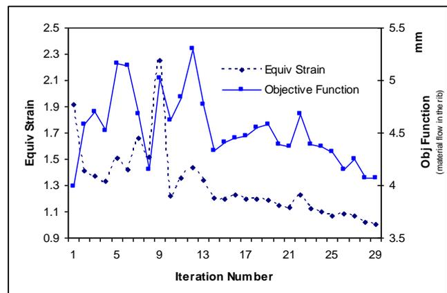
Fig. 6. The Equivalent Strain and Objective Function vs. Optimization Iteration Number
