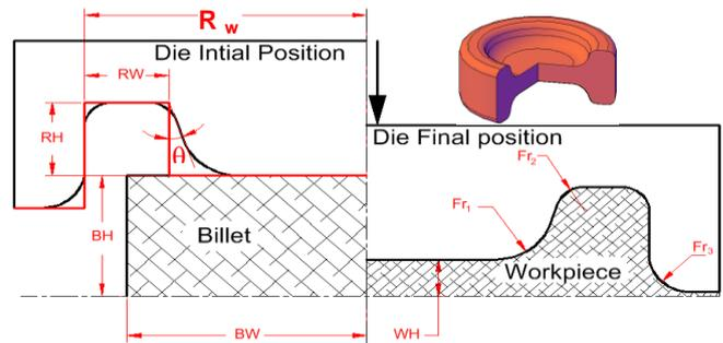
Fig. 1. Configuration of billet and die before and after forging
