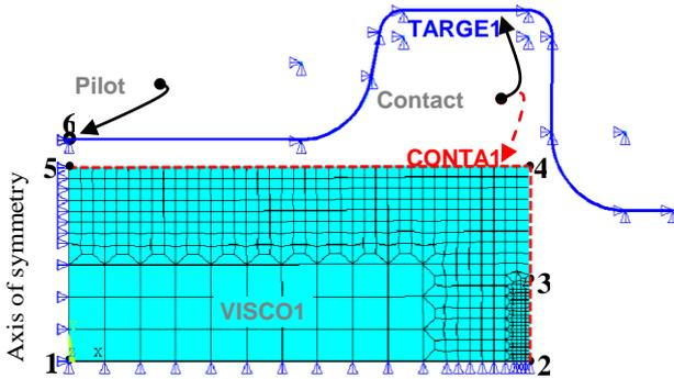
Fig. 3. The discretised model showing boundary condition
