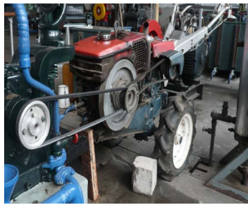
Fig.2. Tractor Coupled to testing equipment
