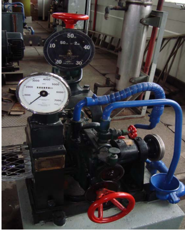
Fig.1. Testing Equipment / FROUDE hydraulic dynamometer
