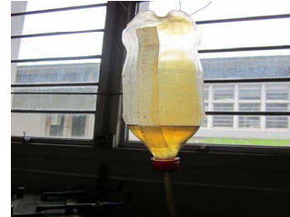
Fig.5. Separate Container for Fuel Consumption Measurement
