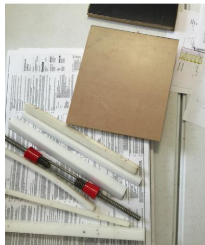
Fig. 9. Formwork samples and Corian insertions for mock-up.
