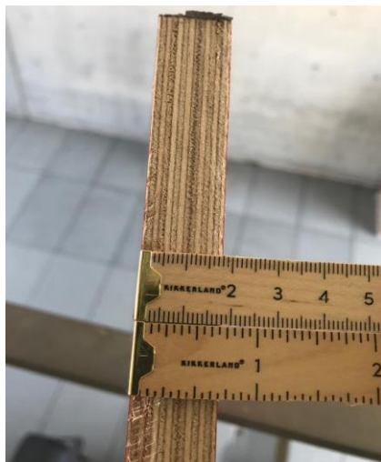
Fig. 5. FinnForm laminated plywood formwork, section detail.
