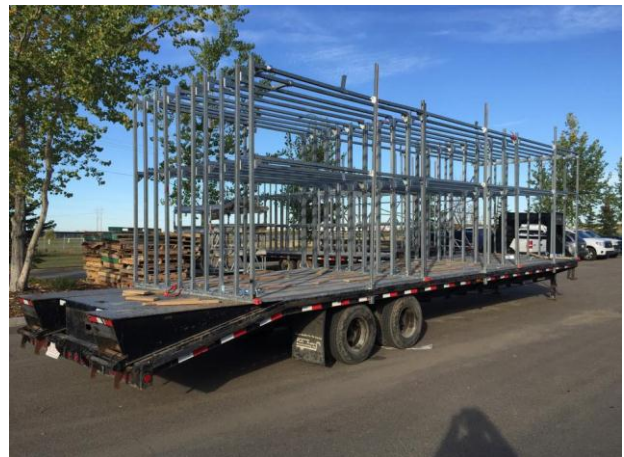
Fig. 9. Special steel frames on trailer for panel transportation.
