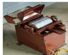
Fig. 2. An Eri Cocoon opener by RuTAG NE, IIT Guwahati.
