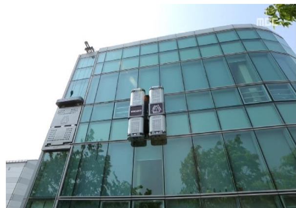
Fig. 1. A window cleaning device developed by Hanyang Univ. [3].
