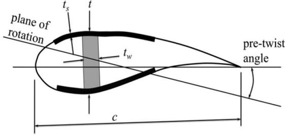
Fig. 4. Blade section diagram.
