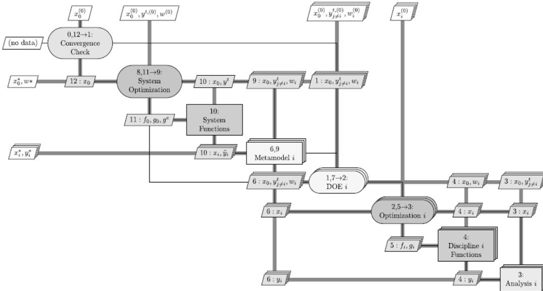
Fig. 3. XDSM diagram for sample BLISS-2000 architecture [18].
