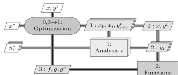
Fig. 1. XDSM diagram for sample IDF architecture [18].
