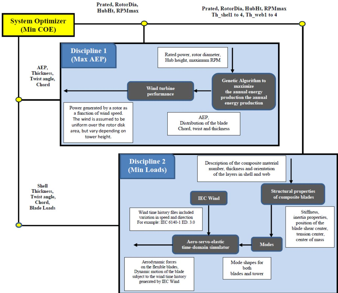
Fig. 5. XDSM for Bi-Level Integrated System Synthesis (BLISS) of the wind turbine deterministic optimization.
