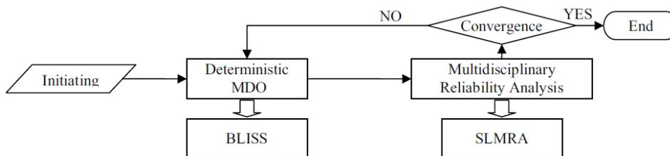
Fig. 6. Procedures of the proposed BLISS-SORA for non-deterministic multidisciplinary design optimization of a wind turbine [4].
