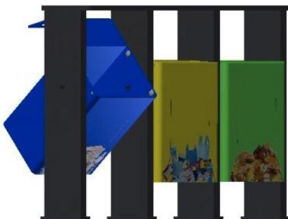
Fig. 8. Swing feature in container.
