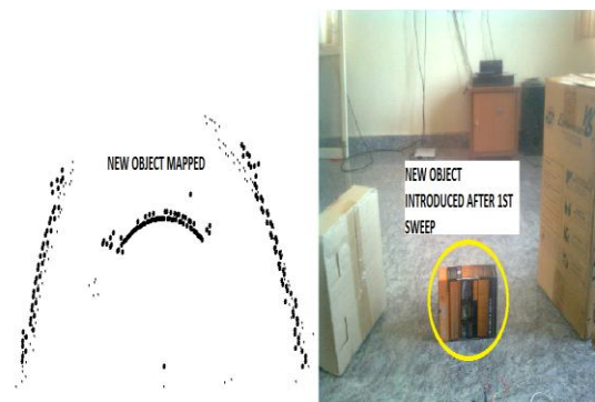
Fig. 6. New object recognized after the 1st sweep during the 2nd sweep.
