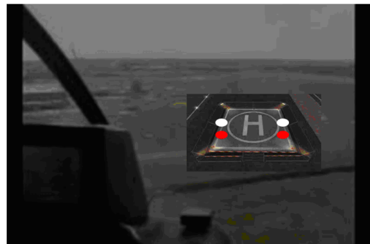
PILOTS WILL KNOW THAT THEY ARE IN CORRECT GLIDE SLOPE WHEN THEY SEE ALL FOUR LIGHTS
