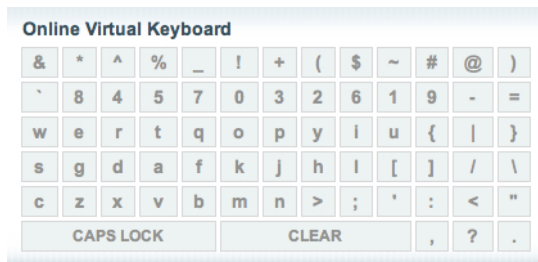
Fig. 11. A typical example of virtual and randomized keyboard as used by State Bank of India in India.
