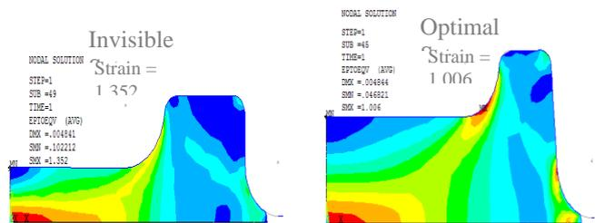
Fig. 5. Effective strain distribution
