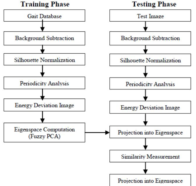
Fig. 4. Block diagram of training and testing phase.
