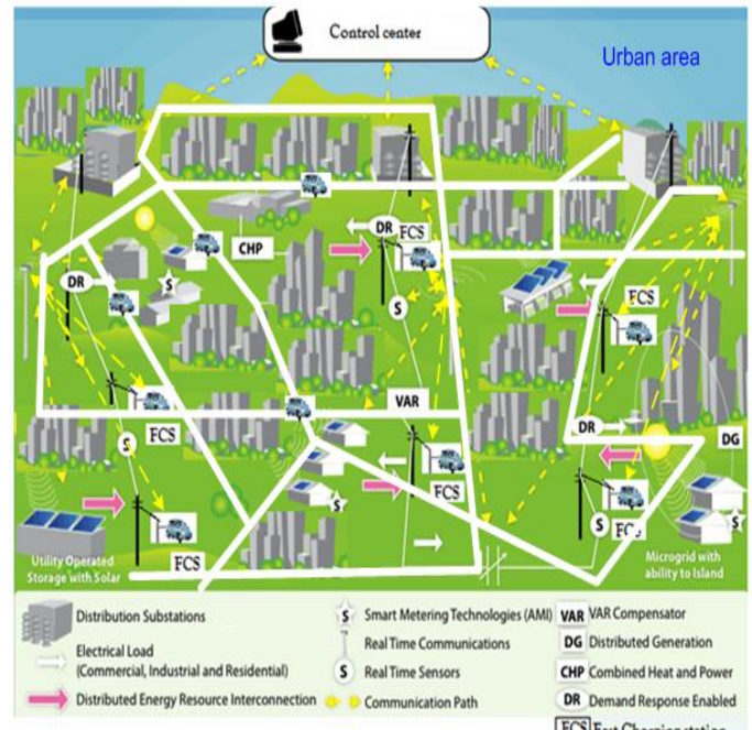
Fig. 5. Proposed smart grid for fast charging station in Thailand
