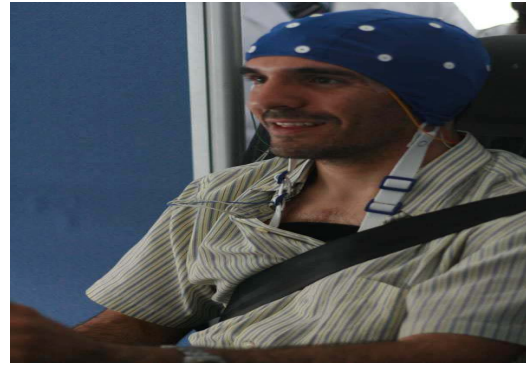
Fig. 2. A driver wearing a helmet with electrodes for EEG.
